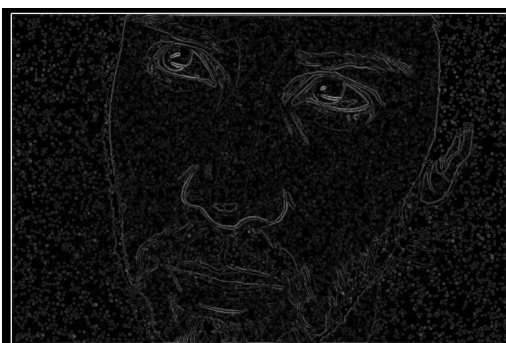
(c) Filter params: Size 6x6, \sigma = 0.75
