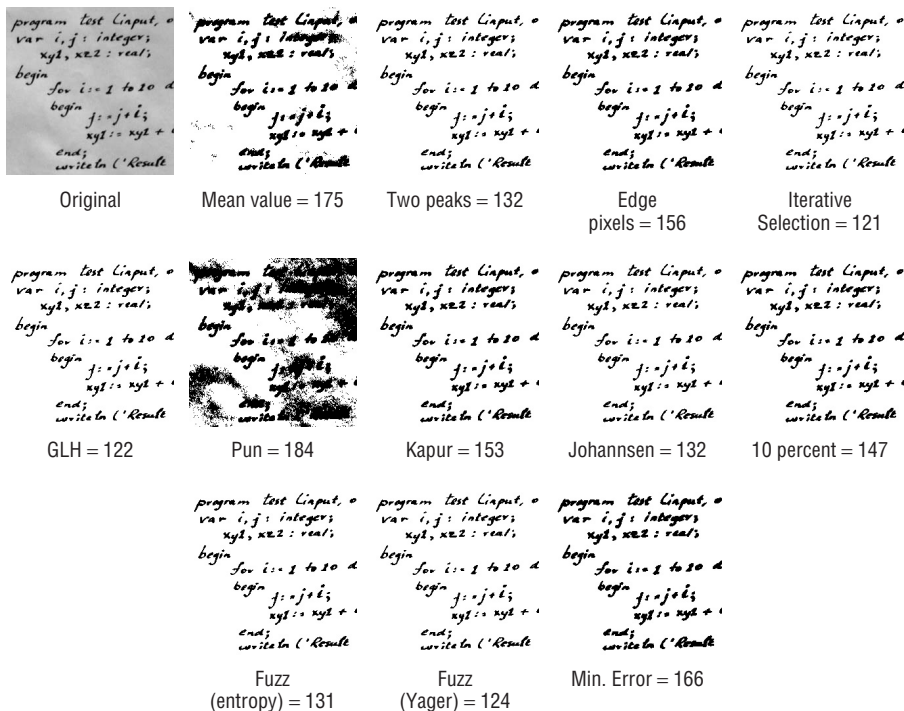
Figure 4.3: Sample results from the single threshold selection methods, using a hand-printed text image (pascal).
