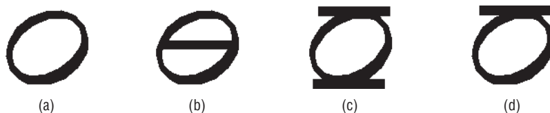
Figure 9.39: Templates for the head of a half note. (a) Basic template. (b) A template for a half note on a staff line. (c) Half note between staff lines. (d) Half note below a ledger line.
