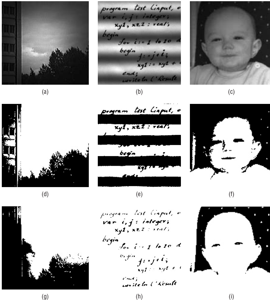
Figure 4.7: Badly illuminated images threshold by Chow-Kaneko and by standard methods. (a–c) The original images with imposed illumination (sky, Gaussian; pascal, sine wave; face, linear). (d–f) The badly illuminated images thresholded using the best thresholding method from the previous trial. (g–i) The same images thresholded by Chow-Kaneko.
